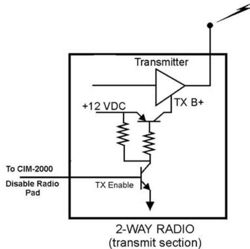
The other method of transmit side disable is to use the Disable Radio Pad (T17) on the back of the CIM-2000. When the CIM-2000 receives a radio kill message, the pad goes low (near ground potential). It stays in this state until a radio enable message is received. Even if the power is removed, (radio turned off) the states are remembered and restored at power-up.
