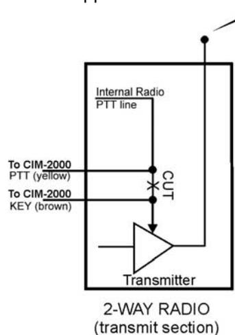
series with the radio keyline. This way, the radio keyline tells the CIM-2000 to key the radio. If the CIM-2000 is in kill mode, it doesn't relay the keying information to the radio. This method requires the keyline of the radio to be broken in order to add the CIM-2000 circuitry in series and "Key Follows PTT" to be enabled in the CIM-2000 programming.
