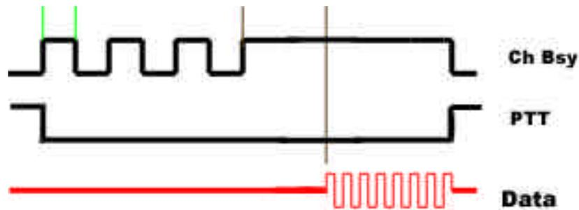
In this timing chart, the distance between green lines is 100mS and between brown lines is 200mS. *Trunk select debounce time* is set for 200mS and *channel busy* input is set for *trunk available when high*.
