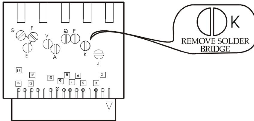
3. **Install** in a radio, with KEY and PTT lines in series with the radio PTT switch.
